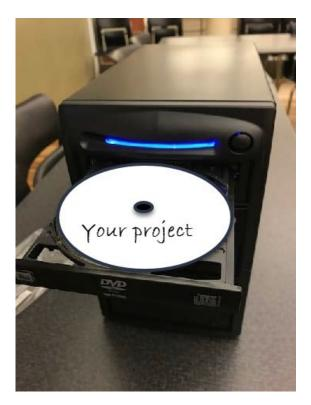
4) Open one of the bottom drives and insert the **<u>BLANK</u>** CD or DVD that is being copied to. There are 3 drives, so you can insert up to 3 blank CDs or DVDs at the same time. Close the drives.
